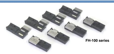
Fiber holder FH-100 series are for Fujikura Fusion Splicer FSM-100 series and FSM-45F/PM series. The FH-100 series has various models depending on coating diameter from  $55\mu m$  to  $1000\mu m$ , and custom one from over  $1000\mu m$  may be available.
